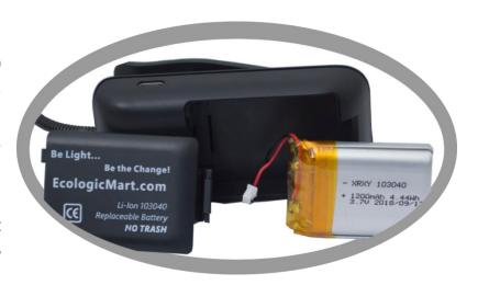
3. Gently insert the battery connector into the receiver at the base, it is important that the red wire is on the left or, the same, the pins are facing up. (please look at the image)
